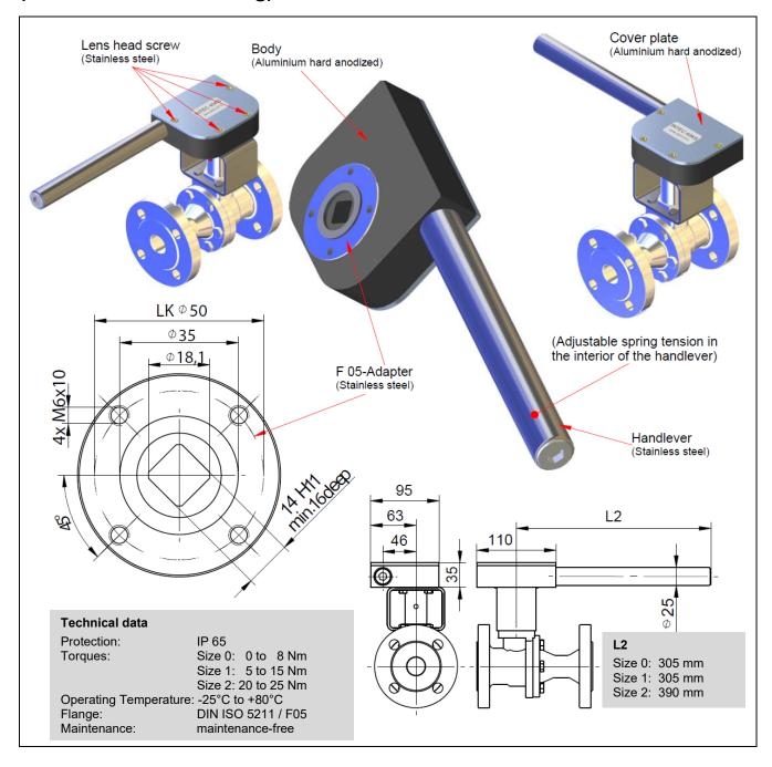
The spring closing unit INTEC 40KS is a user friendly, robust and easy to mounted safety device for all quarter turn valves.
